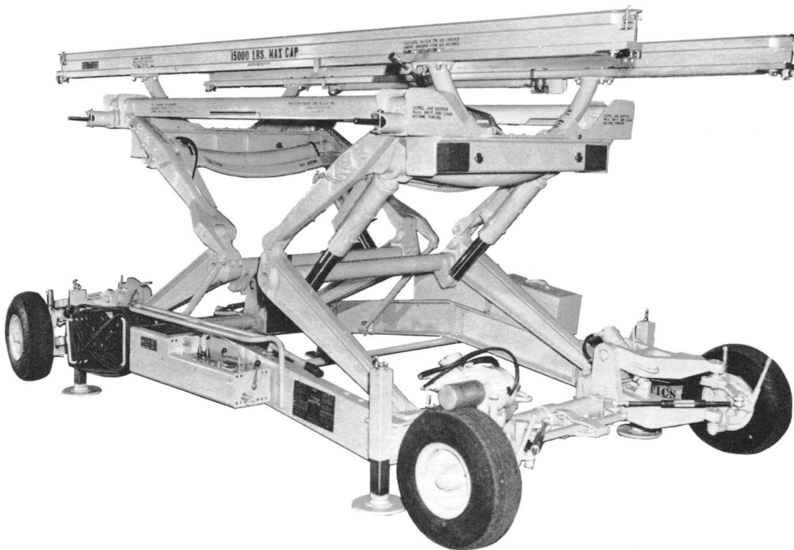
The 15000-pound capacity MODEL 6200 POSITIONING TRAILER shows integral power pack and inching wheel drive
