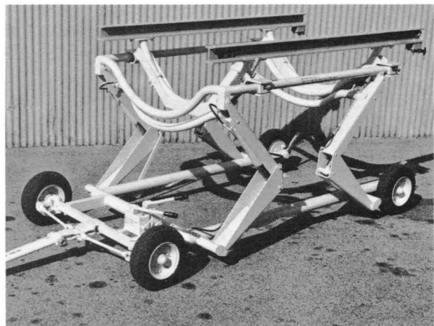
Lightweight, MODEL 1030, positions engines and components up to 3000 pounds.
